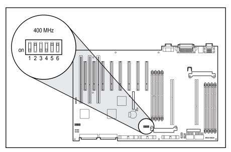
Figure 4-5. 400 MHz processor switch location and default setting
